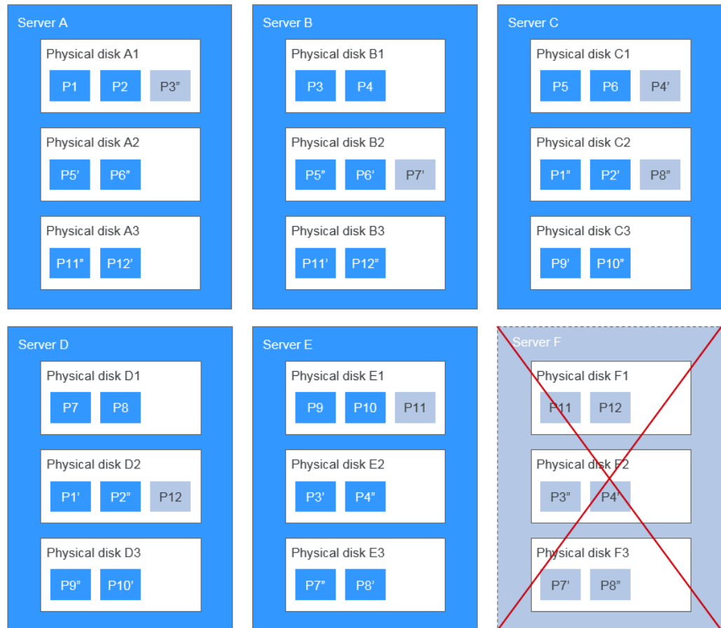
Figure 9-3 Data rebuild principle
